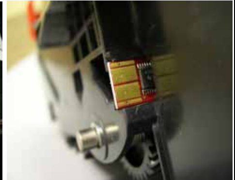
Counterfeit Cartridge w/3 rd Party Chip
